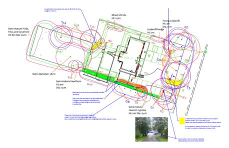
Fig 5: Extract from tree survey showing tree locations
